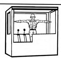
MAGNET IS DISCONNECTED. Crane operator spreads both hands apart, palms up.
