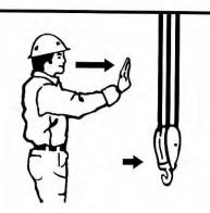
**BRIDGE TRAVEL.** Arm extended forward, hand open and slightly raised, make pushing motion in direction of travel.
